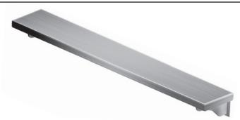
**D.** Work shelf shall be 16 gauge stainless steel. 6" deep with edges turned down square and all corners fully welded, ground and polished. To have #4 satin finish. Support brackets to be stainless steel fold down type.
