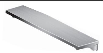
**B.** Solid tray slide to be 16 gauge stainless steel. Ends and side turned down square with all corners fully welded, ground and polished. To have #4 satin finish. Support brackets to be stainless steel fold down type.
