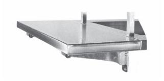
**FF.** End drop shelf to be 16 gauge stainless steel, 30" x 12" wide with edges turned down square and all corners fully welded, ground and polished. To have #4 satin finish. Support brackets to be stainless steel fold-down type.
