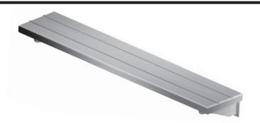
**A.** Beaded 10" tray slide to be 16 gauge stainless steel with two surface beads. Ends and side turned down square with all corners fully welded, ground and polished. To have #4 satin finish. Support brackets to be stainless steel fold down type.
