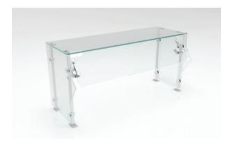
**CCSB.** CCSB models CrystalClear Single Buffet protectors come in standard lengths of 28", 36", 50", 60", 60", 74", 84" and 96". All glass provide is tempered 3/8" glass with pencilled edges and bumped corners. Tubular supports mount on the countertop with two screws through a solid plate on each leg. Options include: heatlamps, heatlamps with lights, and LED lights.
