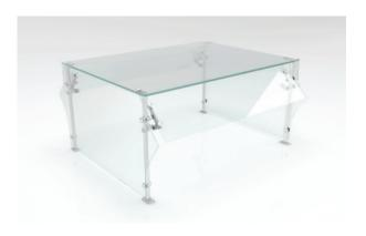
**CCDB.** CCDB models CrystalClear Dual Buffet protectors come in standard lengths of 28", 36", 50", 60", 66", 74", 84" and 96". All glass provided is tempered 3/8" glass with pencilled edges and bumped corners. Tubular supports mount on the countertop with two screws through a solid plate on each leg. Options include: heatlamps, heatlamps with lights, and LED lights.
