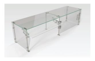
**CCCPADJ.** CCCPADJ models CrystalClear Convertible Counter Protector Adjustable can be self-service or full-service protectors and come in standard lengths of 28", 36", 50", 60", 66", 74", 84" and 96". All glass provide is tempered 3/8" glass with pencilled edges and bumped corners. Tubular supports mount on the countertop with two screws through a solid plate on each leg. Options include: heatlamps, heatlamps with lights, and LED lights.
