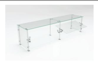
**CCCP.** CCCP models CrystalClear Counter Protector come in standard lengths of 28", 36", 50", 60", 66", 74", 84" and 96". All glass provided is tempered 3/8" glass with pencilled edges and bumped corners. Tubular supports mount on the countertop with two screws through a solid plate on each leg. Options include: heatlamps, heatlamps with lights, and LED lights.
