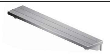
**A.** Beaded 10" tray slide to be 16 gauge stainless steel with two surface beads. Ends and side turned down square with all corners fully welded, ground and polished. To have #4 satin finish. Support brackets to be stainless steel fold down type.
