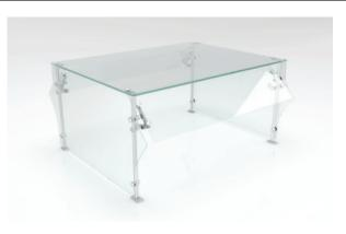
CCDB. CCDB models CrystalClear Dual Buffet protectors come in standard lengths of 28", 36", 50", 60", 66" and 74". All glass provided is tempered 3/8" glass with pencilled edges and bumped corners. Tubular supports mount on the countertop with two screws through a solid plate on each leg. Options include: heatlamps, heatlamps with lights, and LED lights.
