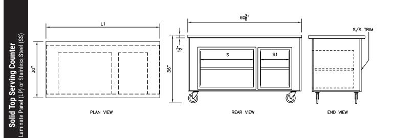
Approx. Ship Weight Model L S **S1** SPC-ST-LP/SS-28 28 3/8" 15" N/A 205 lbs. 36 3/8" SPC-ST-LP/SS-36 15' N/A 220 lbs. SPC-ST-LP/SS-50 50 3/8" 15' N/A 260 lbs. SSPC-ST-LP/SS-60 60 3/8" 28" 15" 300 lbs. SPC-ST-LP/SS-66 66 3/8" 28" 15" 320 lbs. 74 3/8" SPC-ST-LP/SS-74 28' 28' 340 lbs. 84 3/8" 28" 28" SPC-ST-LP/SS-84 360 lbs. SPC-ST-LP/SS-96 96 3/8" 28" 28" 380 lbs.
