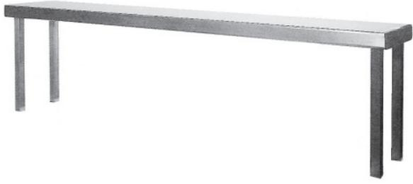
**F.** Overshelf shall be constructed of 16 gauge stainless steel with all edges turned down square and all corners fully welded, ground and polished. To have #4 satin finish. 1" square stainless steel uprights secured to the table top.
